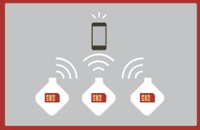
Multiple master devices connect to one target device
